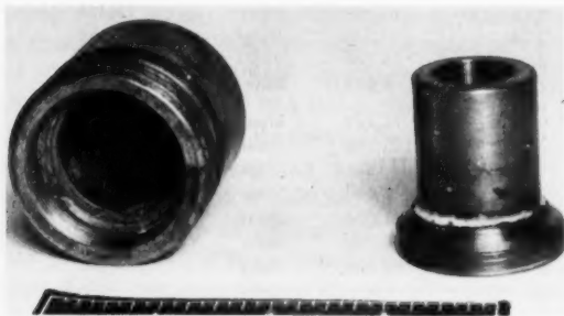
Fig. V-3 Disassembled teletherapy source showing separation of lead gasket. Ruler is marked in inches.
